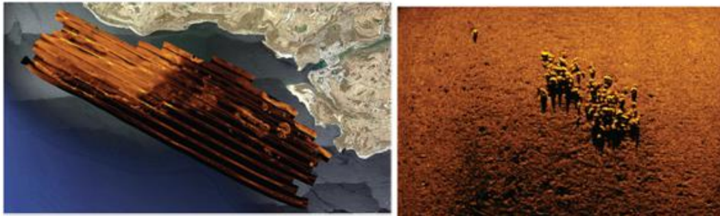
Xlendi wreck, Malta, phoenician wreck 110m deep. Side-scan sonar survey and archaeological target (sonar image in 500kHz) (Gabin et al. 2018, figs. 2 and 3).
